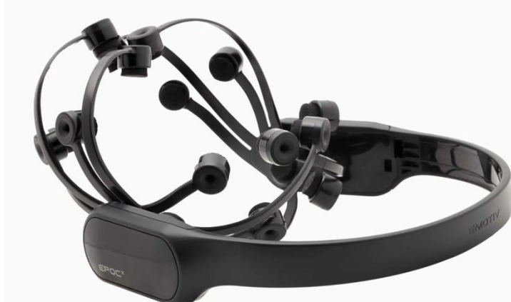
Figure 4: EMOTIV EPOCH EEG device
