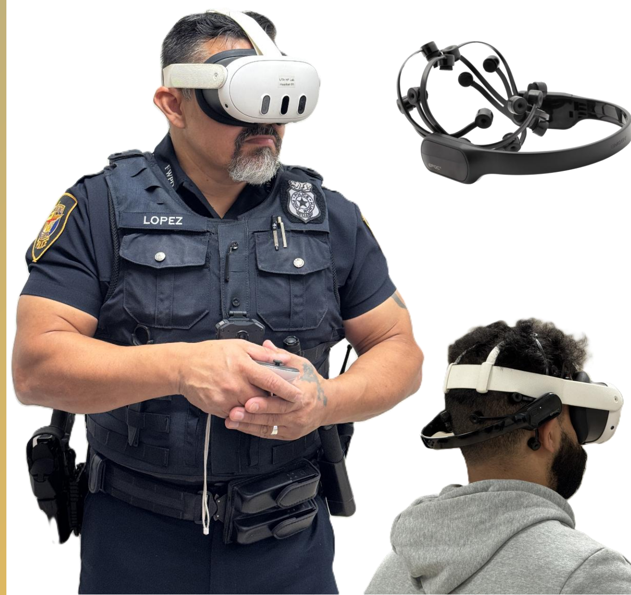
Figure 2. Pilot study measurement setup using VR (Meta Quest 3) and EMOTIV EPOC X EEG recording.
