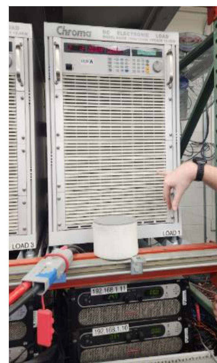
Figure 8. Experimental Devices. The battery connects to the programmable load which is the monitored with a National Instruments card
