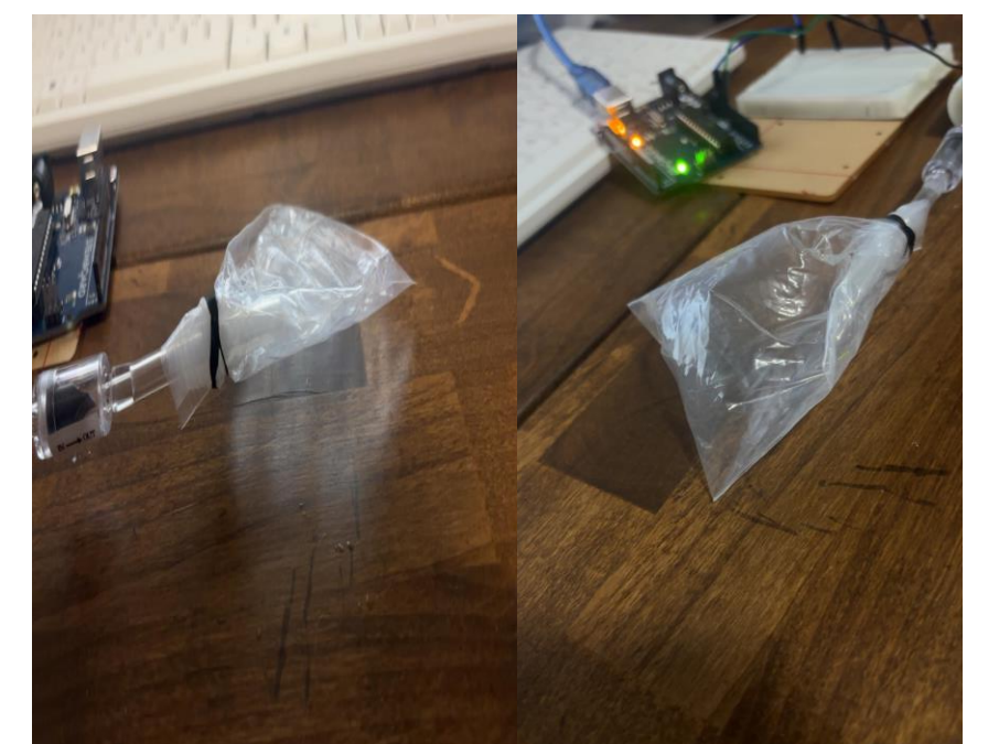
Fig. 6. Dynamic Inflation of Prototype Pneumatic Bladder. Pneumatic Bladder Expansion Demonstration Comparison of the prototype air bladder in its deflated (left) and inflated (right) states during experimental testing. Air delivered by the pump system causes the sealed chamber to expand outward, illustrating the bladder's ability to generate adjustable compression forces that could be used to dynamically modify prosthetic socket fit.
