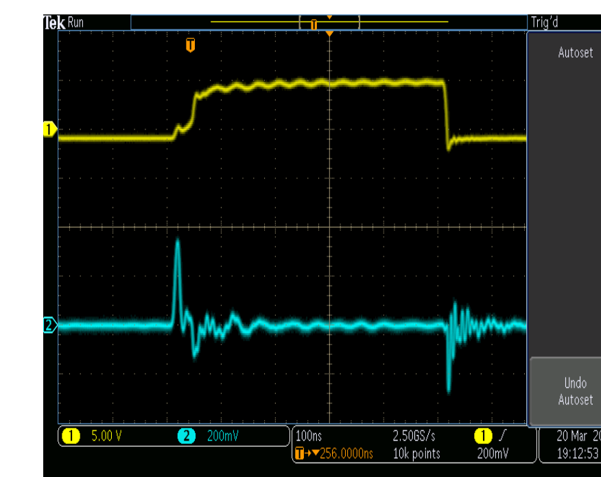
Figure 10: Oscilloscope showed fast switching behavior at 100 ns rise and fall time.
