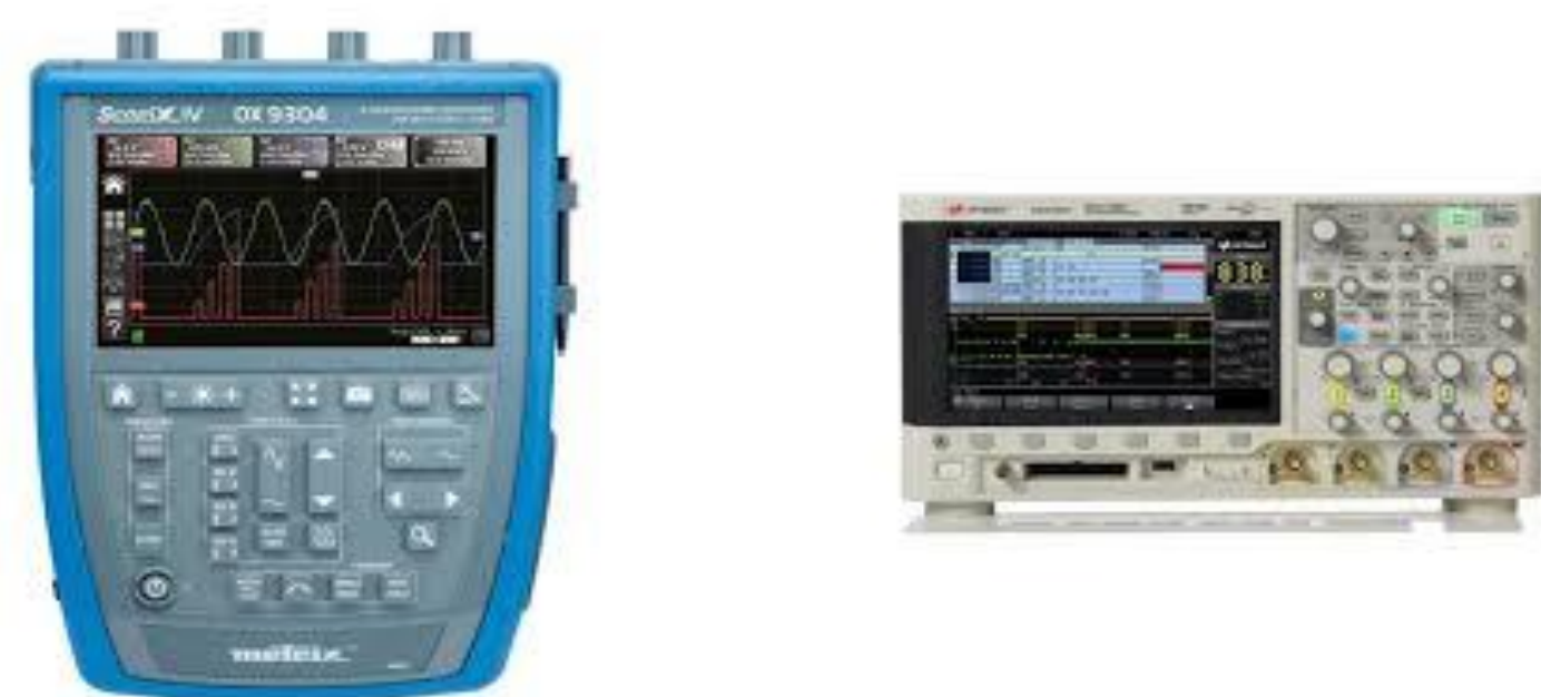
Figure 1. Comparison between Handheld Oscilloscope (Left) and a Benchtop Oscilloscope (Right)
