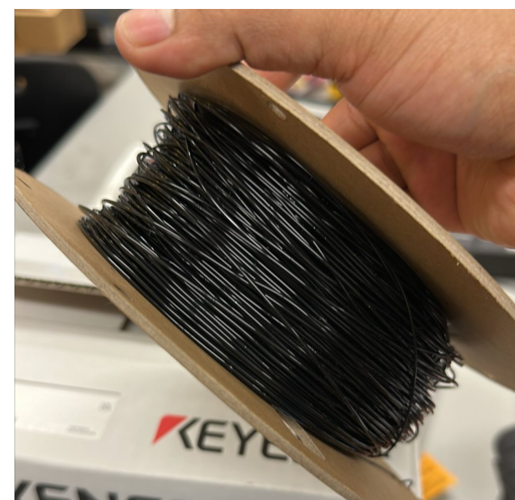
Figure 4: Spooled 1.75 mm diameter filament produced from recycled SLS waste, optimized for use in FDM additive manufacturing processes.
