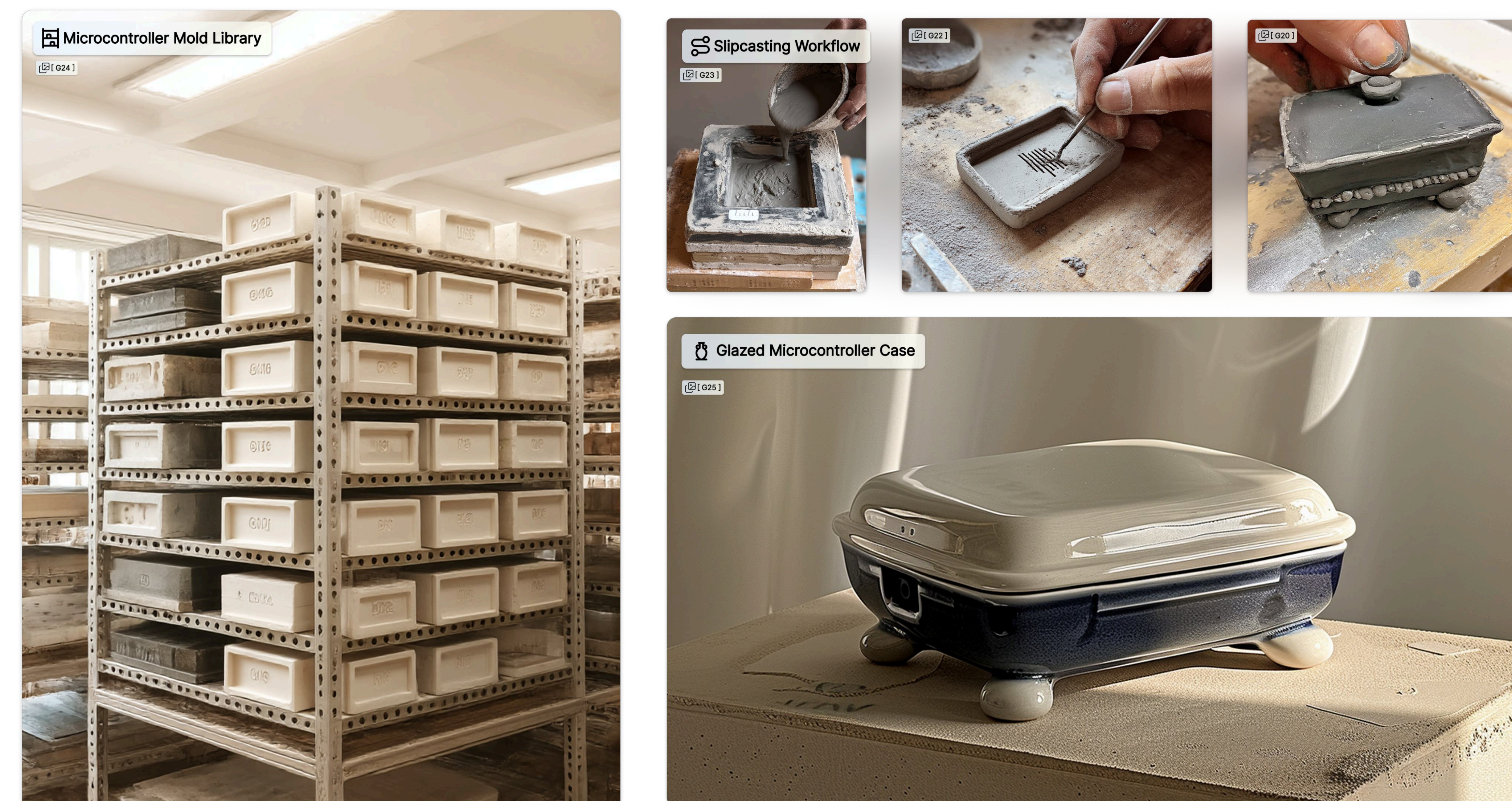
Fig. 1. A speculative ceramic prototyping workflow for microcontroller enclosures. A library of plaster molds accommodating common board form factors enables batch production across varying sizes (left). Slip-cast forms are modified after casting through subtractive carving, additive attachment, and surface deformation (top right). The resulting enclosure is finished with glaze and fired, yielding a durable, craft-inflected housing for embedded electronics (bottom right). (Midjourney v7)
