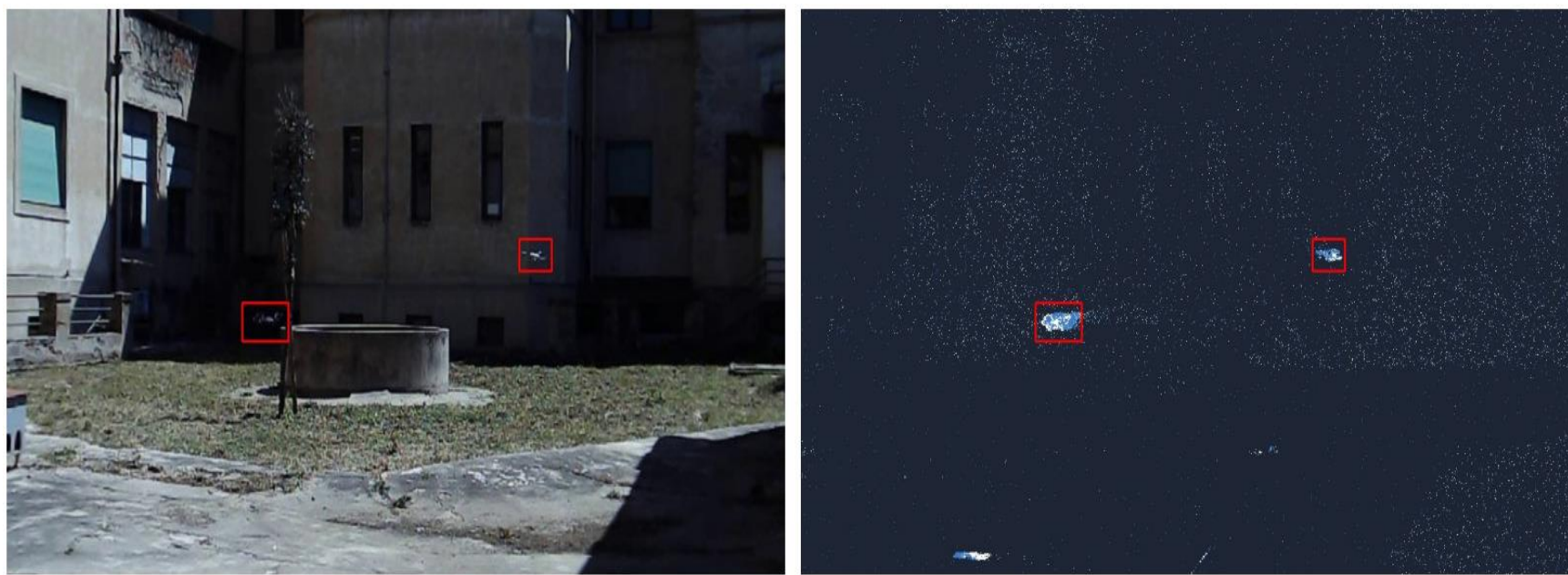
Figure 1. Event cameras pose a paradigm shift in tracking fast moving targets such as UAVs. The left figures are the RGB images, while the right images are the event frames. [1]
